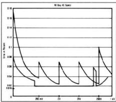
This graph compares the total ac uncertainty of the 8506A's thermal rms converter to that of a typical computing rms converter used in other DMMs. The effects of floor error which cause large uncertainties at the beginning of each range are non-existent in the 8506A from 125 mV ac to 125V ac.
