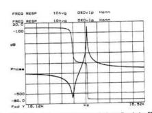
Logarithmic Resolution uses the speed of Linear Resolution FFT measurements to create frequency responses similar to a log-sweep swept sine test. Linear Resolution points are combined internally (rather than just reformatted), on the fly, to create 80-point-per-decade measurements over 1 to 5 decades. Start and stop frequencies can be selected in a 1-2-5 sequence from 0.1 Hz to 100 kHz (for a 0.1 Hz start frequency the maximum stop frequency is 10 kHz — 5 decades).
