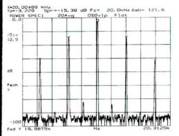
The HP 3562A is essentially a dual-channel spectrum analyzer which provides resolution to 25.6 µHz anywhere within the dc-to-100 kHz measurement range. Single channel accuracy is ± 0.15 dB with 80 dB of dynamic range. Modulation analysis can be performed on either or both channels with harmonic and sideband markers as well as with the built-in demodulation capability: zoom measurements can be AM, FM or PM demodulated with carrier frequencies up to 99.9 kHz.
