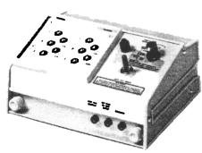
One of the features that sets the 576 apart from the 577 is the display area READ-OUT. Adjacent to 576's crt are alphanumeric indicators of vertical and horizontal deflection factor, step amplitude, and Beta/div or gm/div. The Beta or gm readout saves the operator from the arithmetic usually necessary to arrive at these parameters. The READ-OUT also provides a permanent record of major knob settings in 576 crt photographs.
